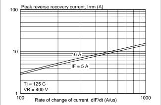
Fig.8. Typical peak reverse recovery current, I<sub>rm</sub> as a function of rate of change of current dI<sub>E</sub>/dt.
