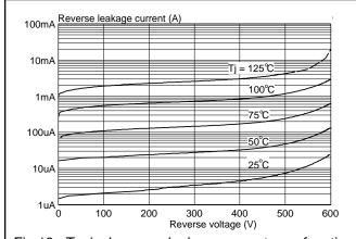
Fig.13. Typical reverse leakage current as a function of reverse voltage.  $I_R = f(V_R)$ ; parameter  $T_j$
