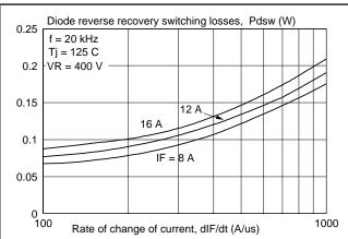
Fig.4. Typical reverse recovery switching losses in diode, as a function of rate of change of current dl<sub>F</sub>/dt.
