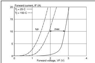
Fig.12. Typical and maximum forward characteristic  $I_F = f(V_F); T_i = 25 ^{\circ}C \text{ and } 150 ^{\circ}C.$
