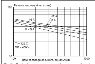
Fig.7. Typical reverse recovery time  $t_r$ , as a function of rate of change of current  $dl_r/dt$ .
