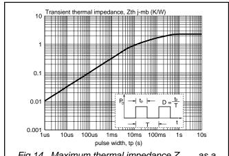
Fig.14. Maximum thermal impedance  $Z_{th j-mb}$  as a function of pulse width.
