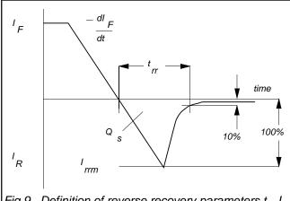
Fig.9. Definition of reverse recovery parameters t<sub>rr</sub>, I<sub>rrm</sub>
